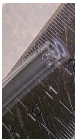
Application specific automatic machine that cuts and punches tubes. Tube length can be adjusted, as well as hole diameter upon changing punching tool. Actual hole diameter is less than 2 mm.
